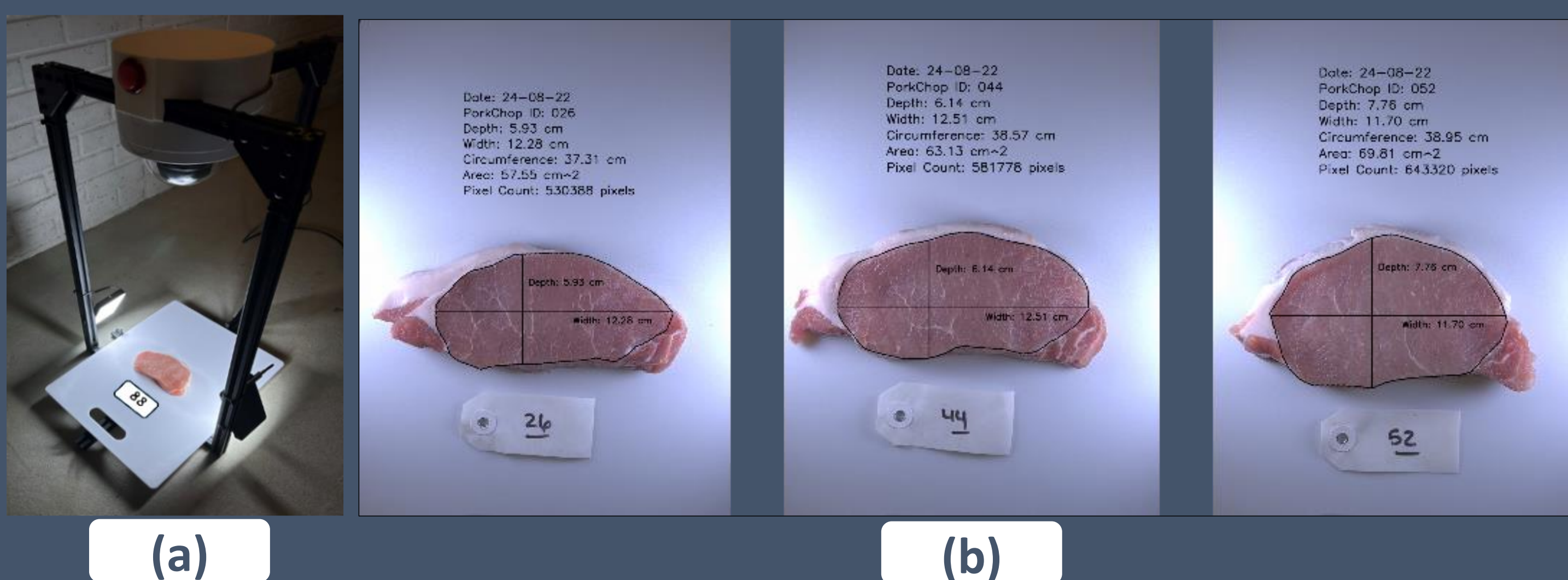
Figure 1. Device used for image capture (a) and three visualizations of pork chop size estimation (b)
