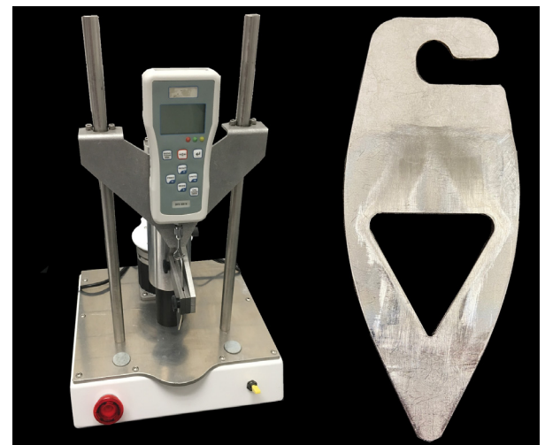
Figure 3.12 Warner-Bratzler machine and blade
