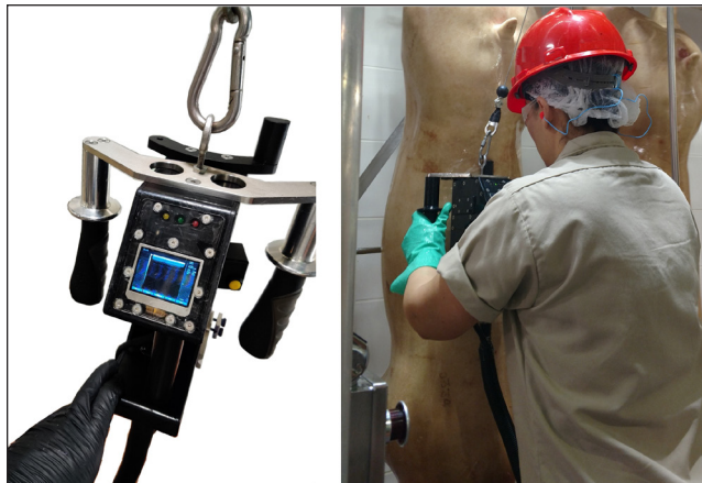
Figure 1.7 Ultrasound carcass grading instrument
