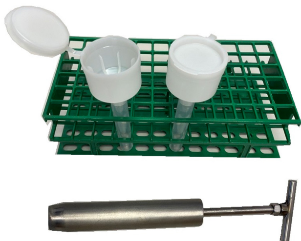
Figure 3.9 EZ drip loss tubes and coring device
