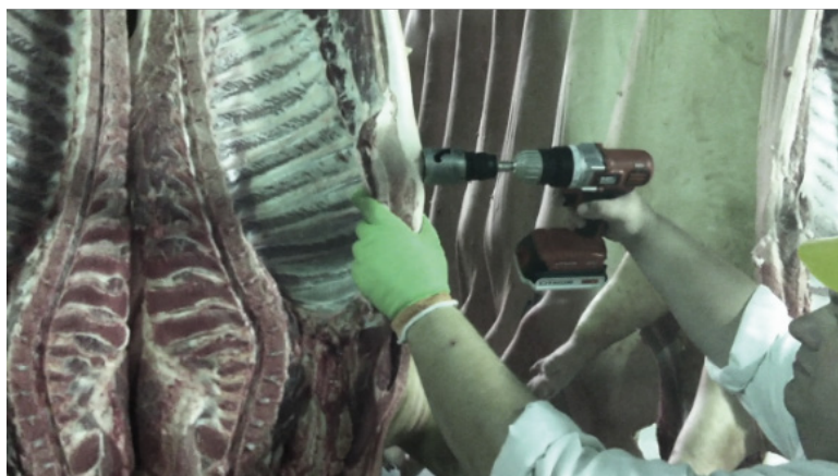
Figure 4.1 Coring device mounted on a drill to collect fat samples
