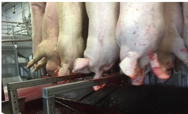
Figure 3.25 Use of head knockers to prevent blood clotting
