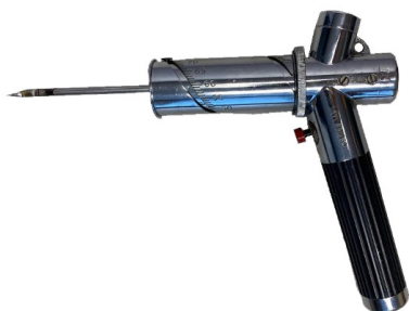
Figure 1.3 Intrascoper used for measuring backfat thickness
