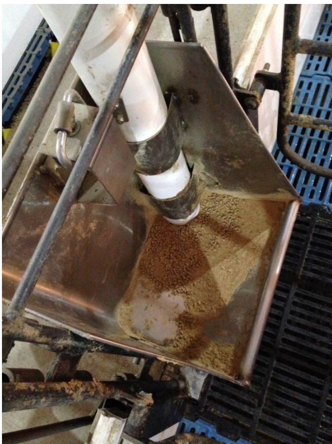
Figure I8. Correctly Adjusted Lactation Feeder with Fresh Feed
